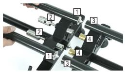
Tighten the mounting screws.
