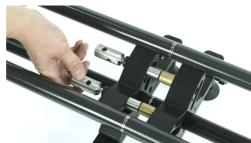
It is easier to assemble the sections with a special key [1], which allows to tighten the screws with more force.
