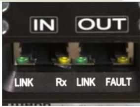
If the backlight of the LCD screen starts flashing and there will be an orange flashing light under FAULT marking on the right socket of the driving motor, the user is informed about existing error. In such situation, immediately enter CONFIG menu → [Info]. Information about the error should appear in the upper right corner of the screen.
