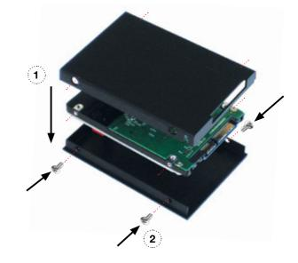
(1) Important: Insert screws last and DO NOT over-tighten the screws or proper alignment of the Master Caddy can not be guaranteed.
